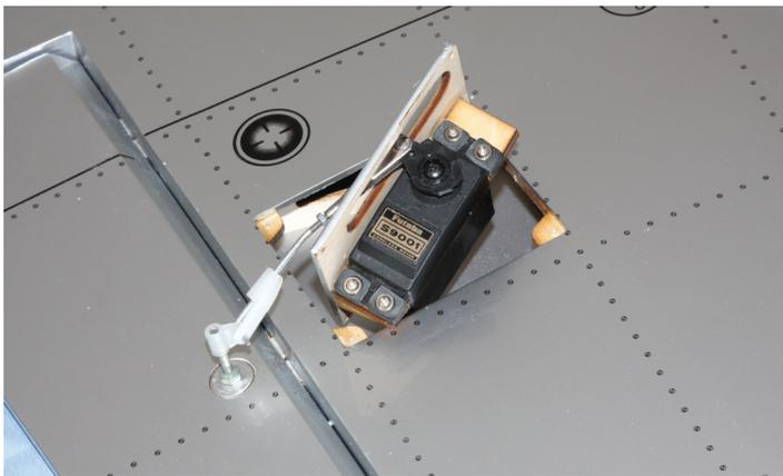
*A standard size servo fits neatly into the aileron servo box*
