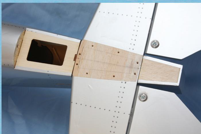
Remove film covering from this area to adhere the fin seat
