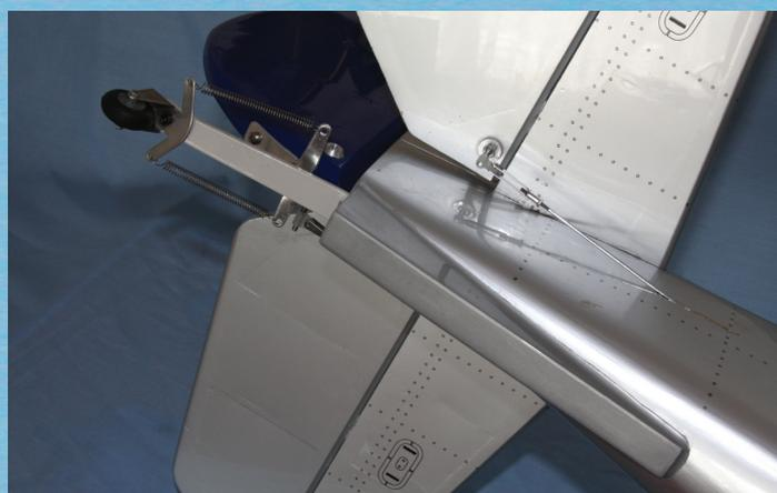
Steering tailwheel assists ground control; note the scale moulded covering over the tailwheel bracket
