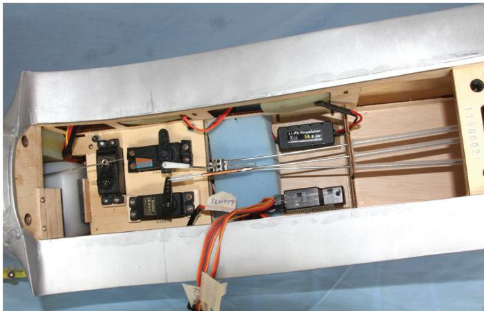
*A neat radio installation, but I had to extend the rudder pushrod (see text)*
