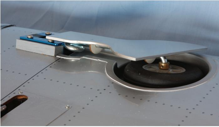
*Main retract unit is raised from the wing to give it the correct rake angle and does not deter from the operation or flying*
