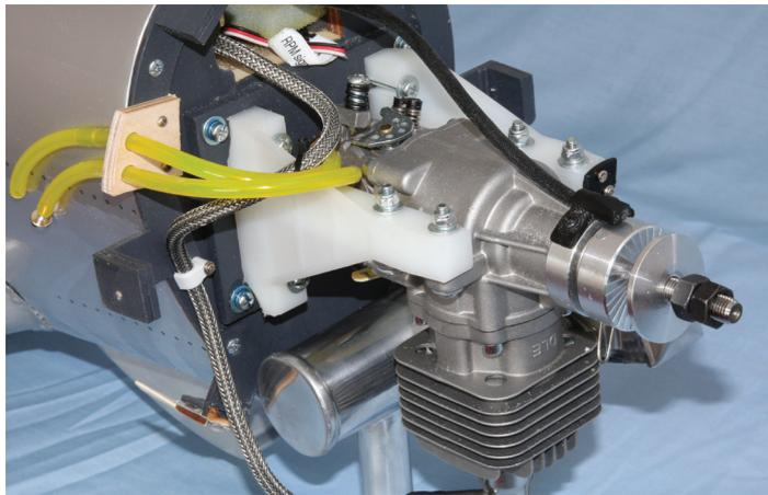
*The powerplant chosen was the DLE 20 cc petrol, which required a little modification to the firewall but the space inside the cowl is ample*
